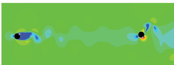
(e)  $S/D=20$ 图 6  $Re=44\ 450$  时串列双圆柱尾流结构Fig. 6 Wake structures for two cylinders in tandem arrangement at  $Re=44\ 450$
